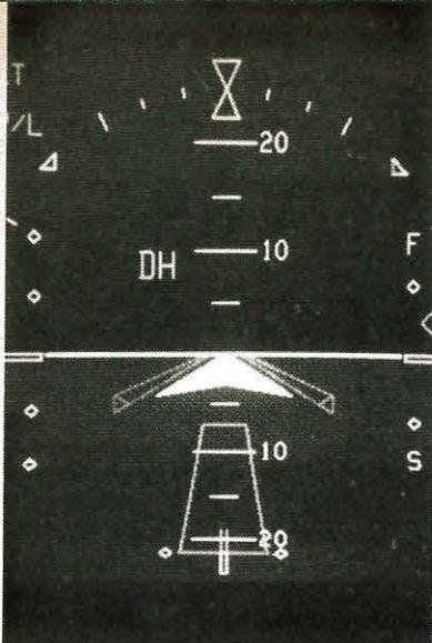
**Cover image:** A 5" x 5", color avionic CRT display tube achieves its high resolution through the use of a fine 0.2 mm pitch shadow mask and very rugged in-line electron gun. Innovative self-converging deflection system, static color purity with convergence correction, and an effective contrast enhancement filter contribute to the very bright display. *AEG Corp., Somerville, NJ.*
